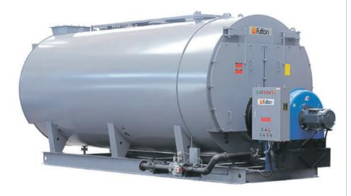
FB-C boiler is designed and manufactured to comply with ASME code and Chinese boiler Standard, with standard maximum working pressure of 1.0 MPs (150 PSI) or 1.25 MPa (185PSI). The standard model is three pass, wet back, and corrugated furnace. The factory also supplies 4-pass. wet back corrugated furnace boiler or higer pressure boiler upon customer's request.
